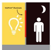
ViziPrint<sup>®</sup> Illuminate is a 4 mil (100 $\mu$ ) high quality, translucent matte PET film that uses a mechanical bond to adhere graphics to glass and other smooth, flat surfaces. Thanks to its proprietary adhesion technology, no adhesive residue is left behind during graphic removal.
