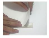
5. Remove the liner on the front tape and press the graphic on the panel strip. Do the same to the top panel strip (squarely).
