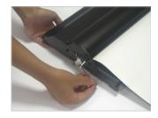
8. Put the graphic roller back into the base and secure the lid on both sides with the hex key.
