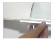
7. Insert the top panel strip into the top profile. With a piece of clear tape on the back, center and secure the graphic to keep it from sliding.
