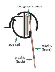
5. Fold the top of the new graphic backwards once and then slide into the top rail.
