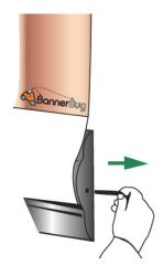
6. While carefully holding the graphic, remove the pin from the side of the system and gently allow the graphic to roll back into the unit.
