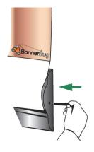
1. Release the graphic panel completely from the system to expose the PVC tongue and graphic join. Place the pin into the side of the unit when the hole on the roller lines up with the hole in the end cap.
