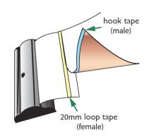
2. Carefully remove the existing graphic panel from the PVC tongue. Add 0.78" (20mm) hook tape (male) to the base of the new graphic panel and then place in the same position.
