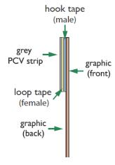
4. Add 0.63" (16mm) hook tape (male) to the top of the new graphic panel and apply the existing grey PVC strip.
